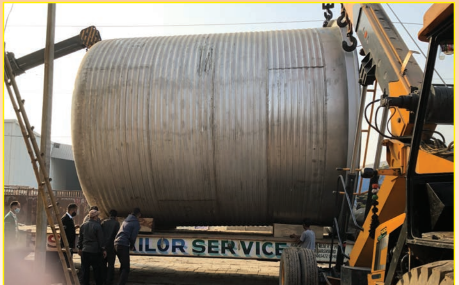
Inner Cover / Retort of 4800 mm ID x 7000 mm Height
