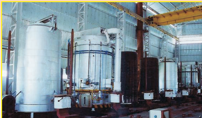
80 Ton Bell Type Bright Annealing Furnace
