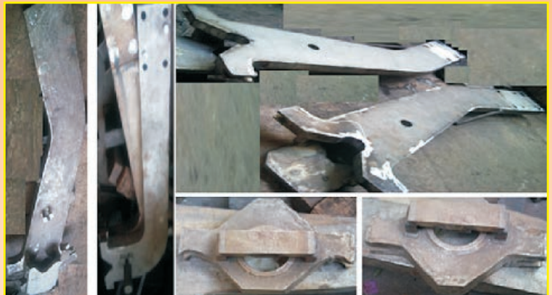
SS 316 L Grade Fabricated Sink Roll and Stabilizer Roll Arms and Bush Housings for Rolls of Galvanising Line.
